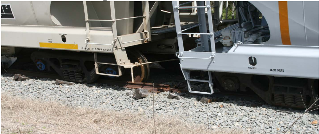
Figure 4 – Cars off the rail on a siding in Commerce, Texas due to severely Deteriorated Crossties that contribute to Gauge Variances.
