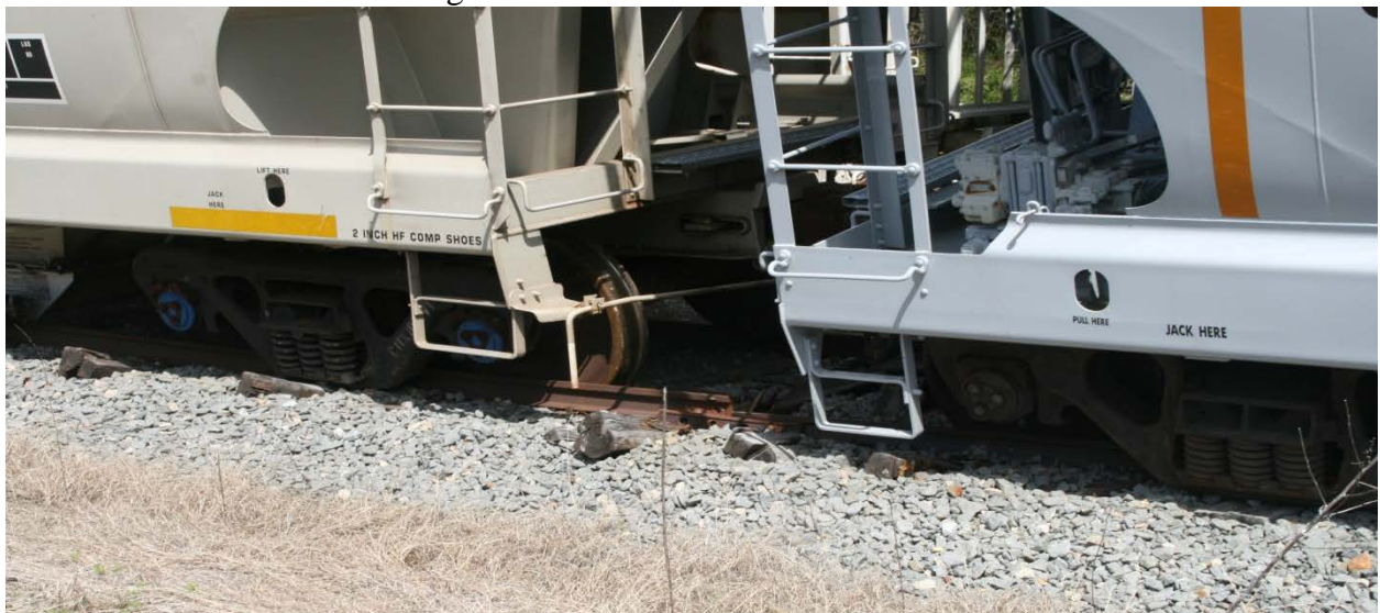
Figure 4 – Cars off the rail on a siding in Commerce, Texas due to severely Deteriorated Crossties that contribute to Gauge Variances.
